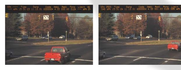
tween the pictures can be set within a range from 1/2 to 10 seconds. Alternatively, the operator may determine the position of the car on the second photograph.
